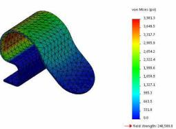
Using SOLIDWORKS Simulation Professional software, CamelBak quickly optimized the leaf-spring design for the auto-seal trigger mechanism on the Forge insulated travel mug, improving performance, reducing prototypes, and securing a patent for this product innovation.
